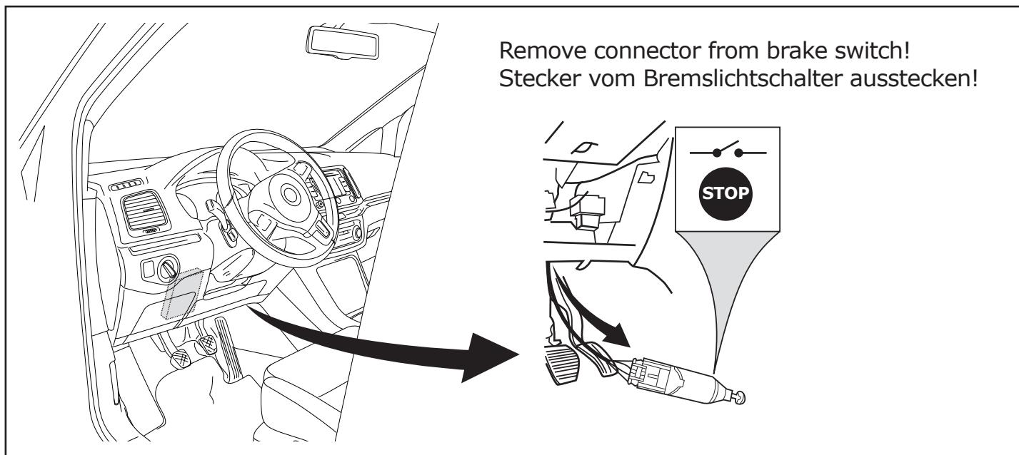
Remove connector from brake switch!
